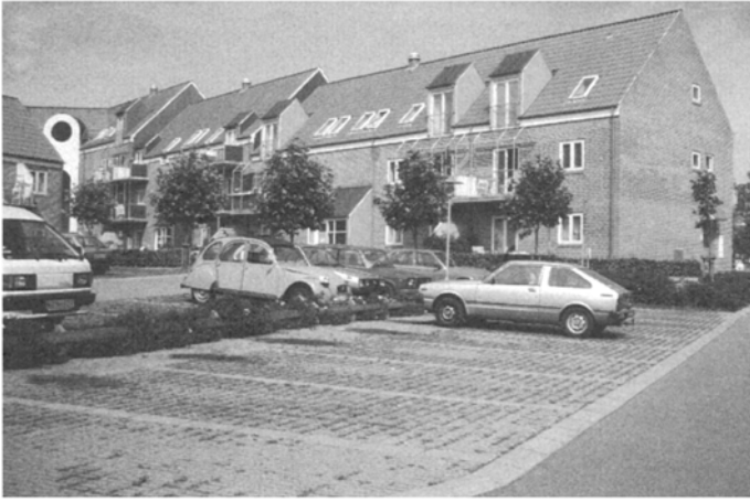
Fig. 12. Grasscret™ pavers are used in residential parking in Aarhus, Denmark.
